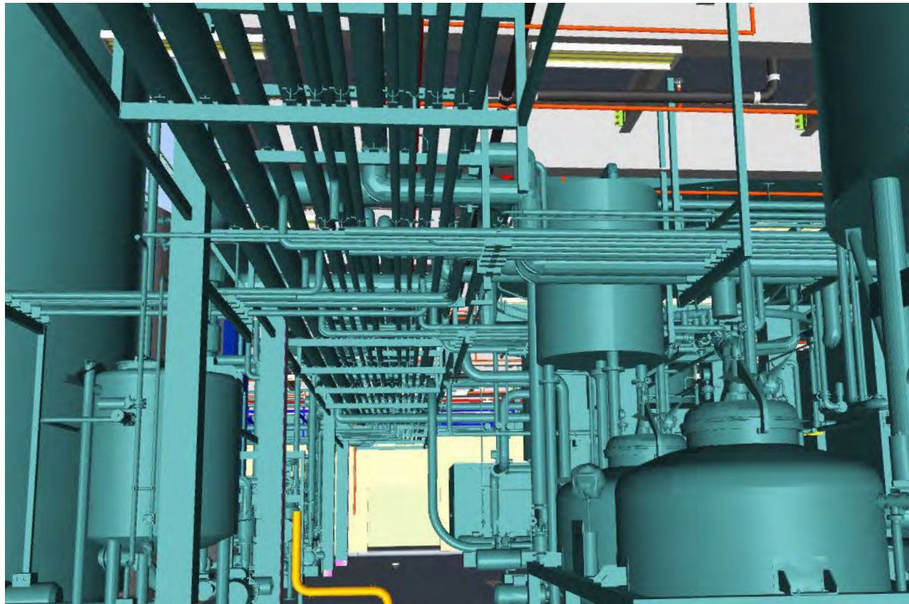
Design coordination through the development of a 3D model with base building criteria, process points of connection, and MEP points of connection were crucial to the design and development of the brewing process. This image shows the pipe bridge over which a second level tour path will allow employees and visitors alike to look over the production, packaging, and distribution processes.
